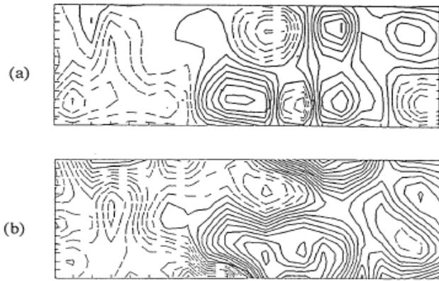
Fig. 8 The contour of the distribution of the vertical velocity in a horizontal plane near the river surface. Depth from the surface ; (a) -0.2m ; (b) -0.6m
