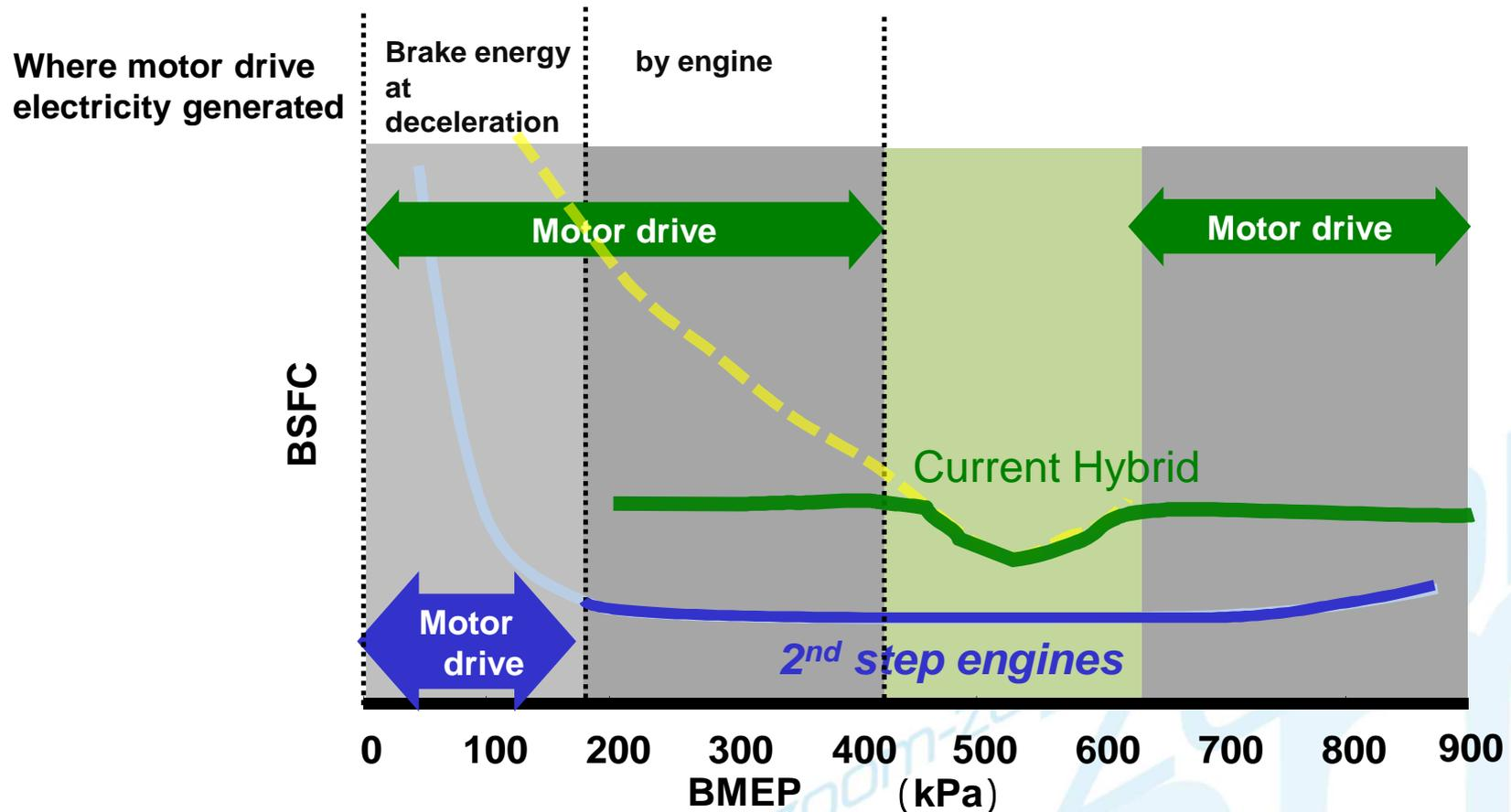
When Mazda's next-generation engines are hybridized, small-sized motor and battery are sufficient enough to power engines.
