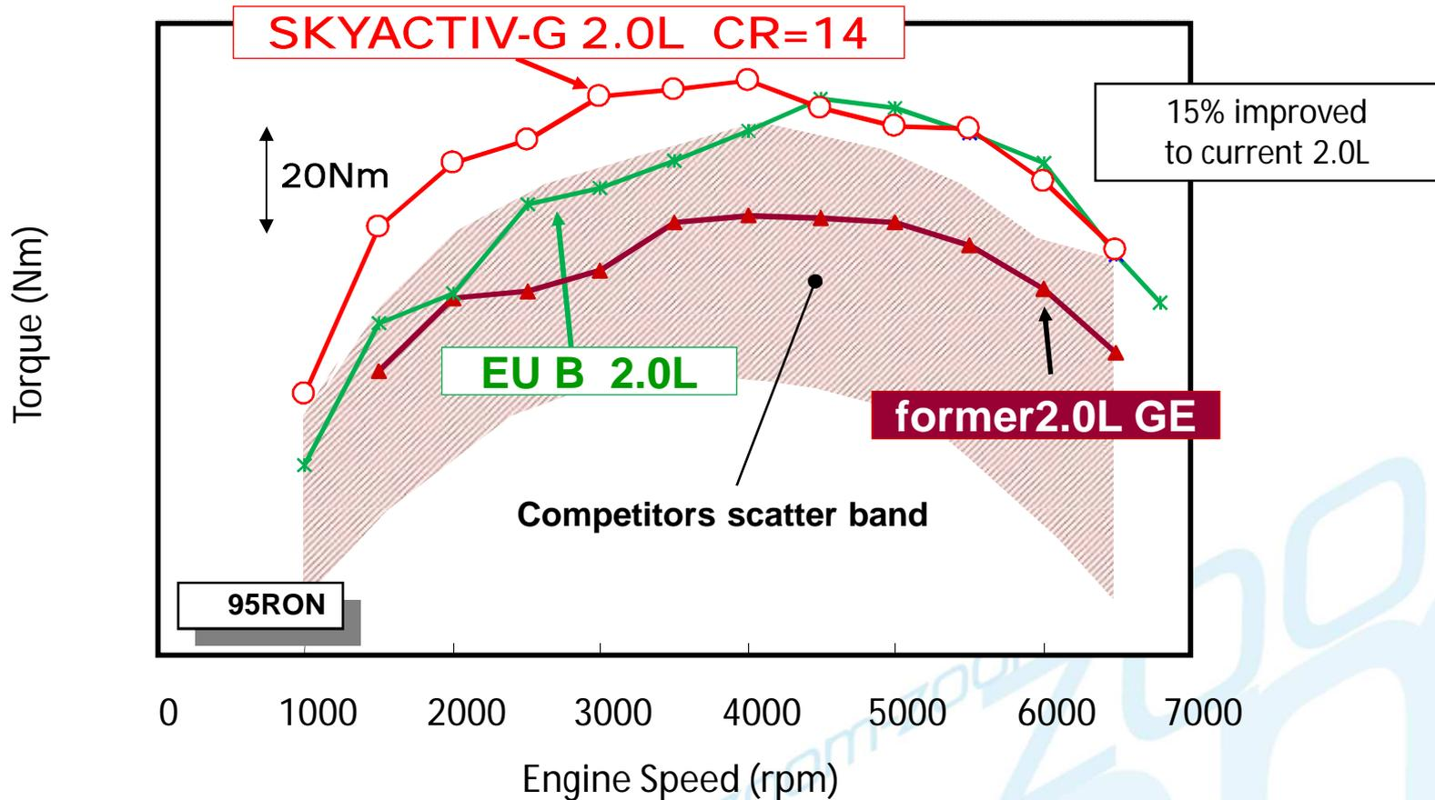
Improve low- and-mid end torque in spite of a high compression ratio and achieve superior driving
