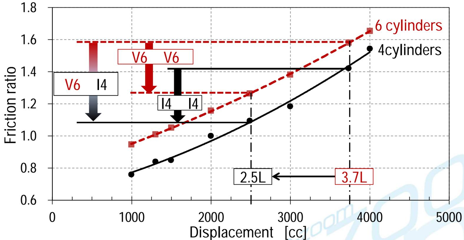
Mechanical friction reduction due to downsizing 3.7 L V6 to 2.5 L I4 is 1.6-times greater than downsizing 3.7 L V6 to 2.5 L V6 or 3.7 L I4 to 2.5 L I4. As a result, fuel economy is significantly improved.
