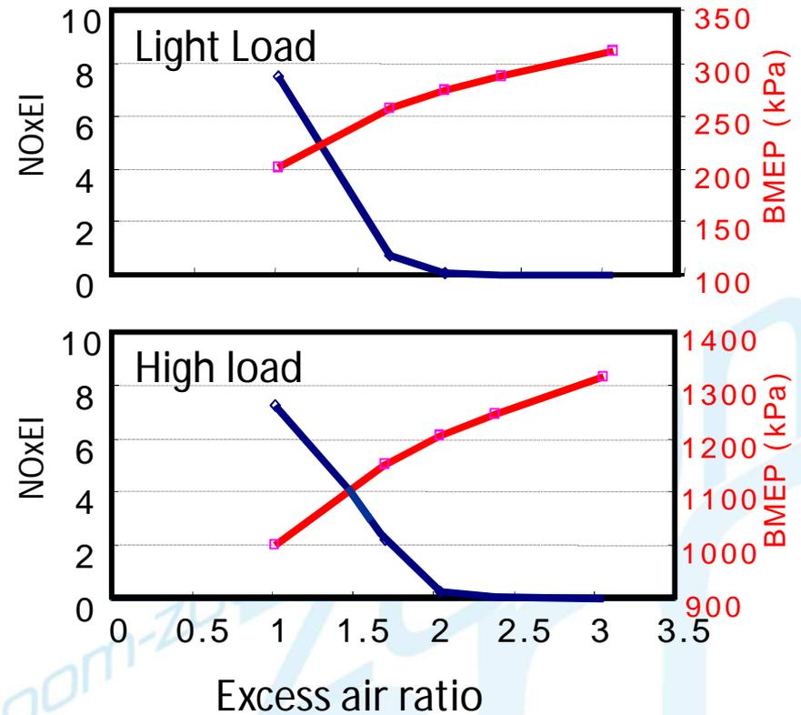
Expanding  $\Lambda > 2.2$  is required for the compatibility of both efficiency and no NOx after-treatment
