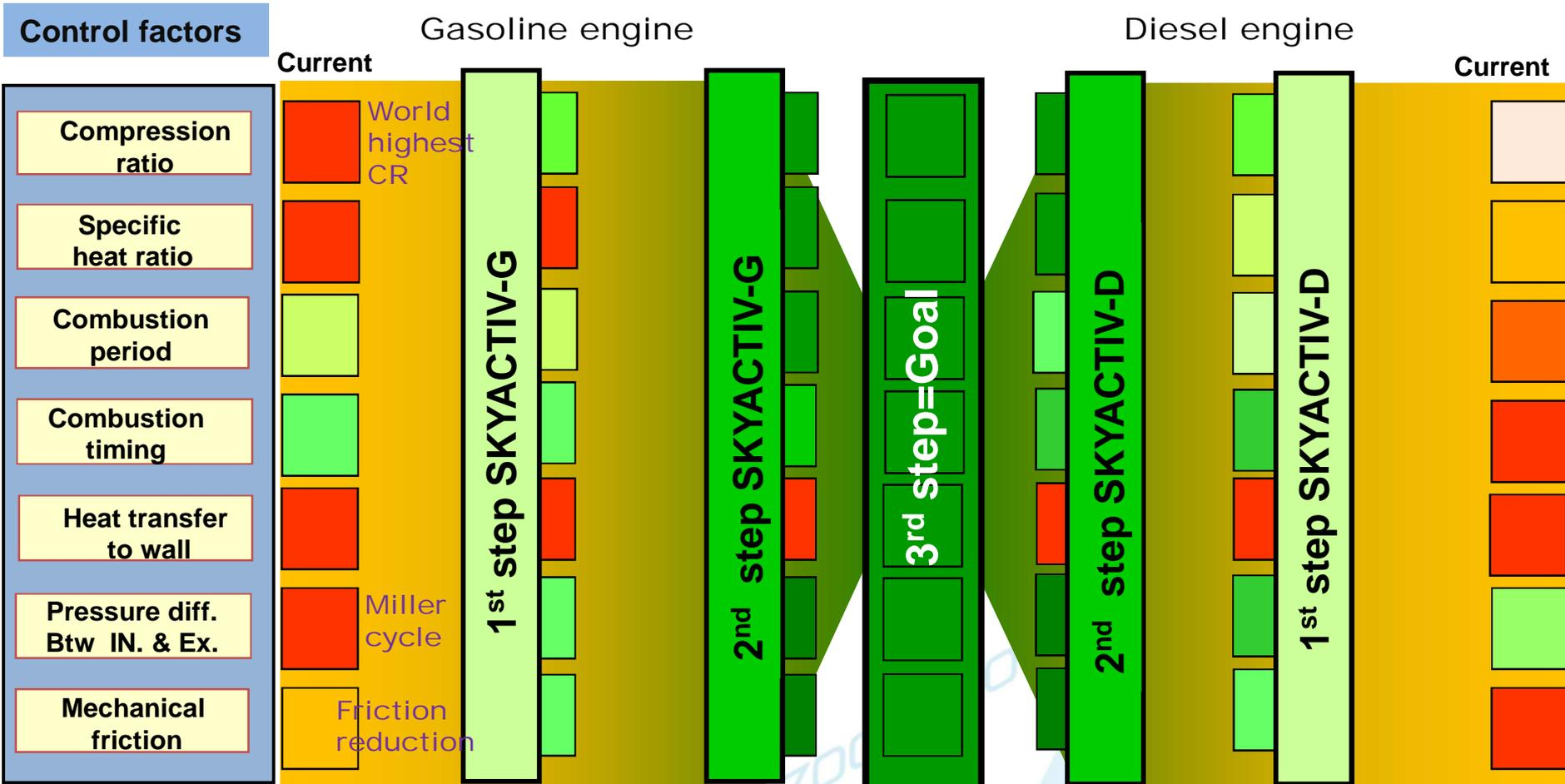
The most distinctive feature of 1<sup>st</sup> step gasoline engine is world highest compression ratio.
