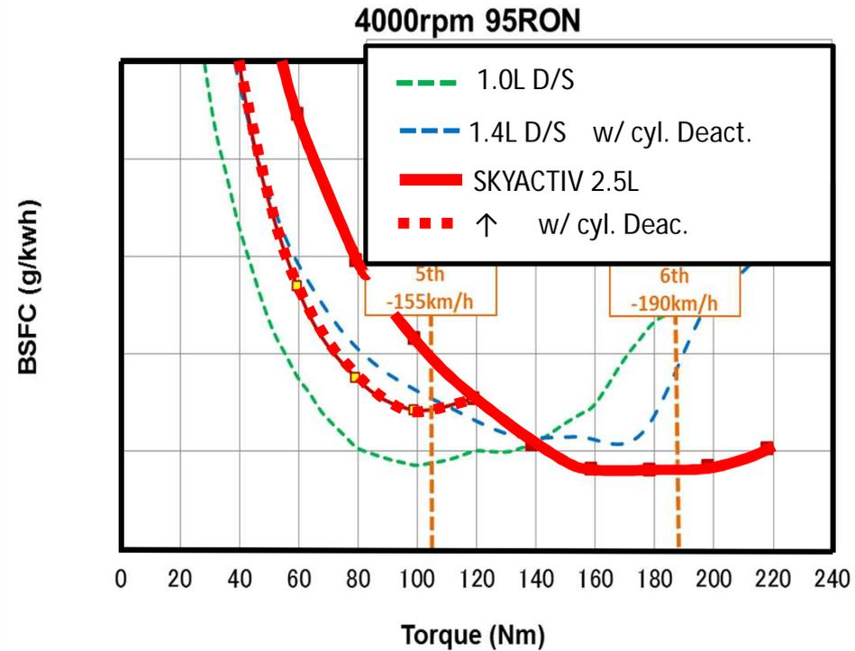
Even 2.5L SKYACTIV engine can be superior to 1.4L 4-cylinder boosted D/S engine with a cylinder deactivation system, and 1L 3 cylinder boosted D/S engine in all operational ranges.
