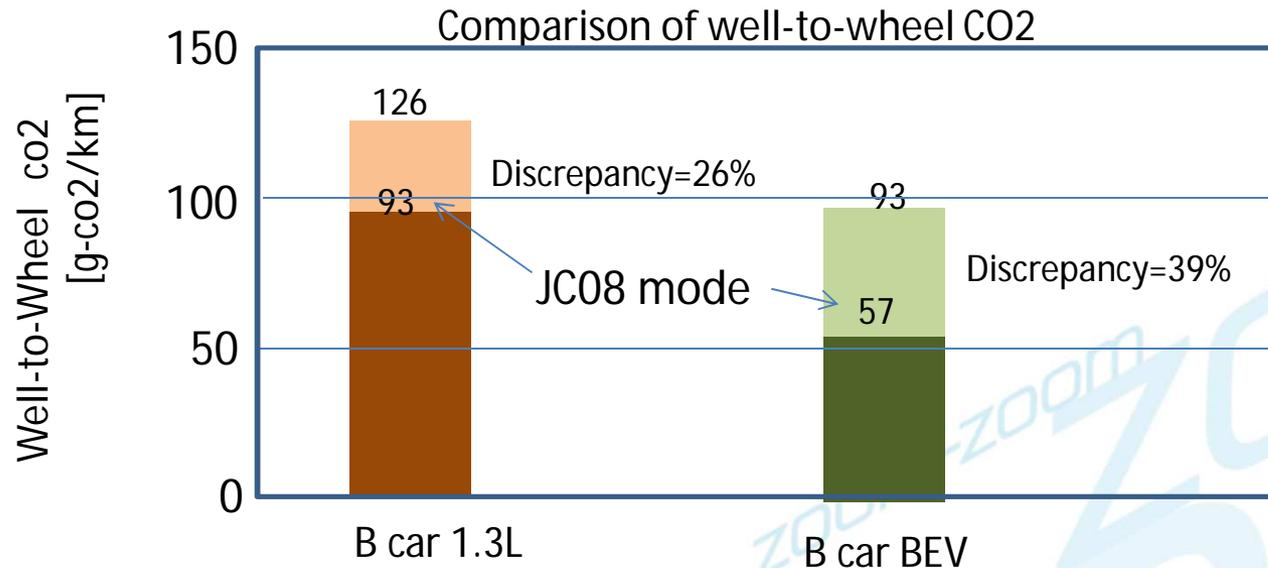
Fuel economy of internal combustion engines needs to be reduced by approx. 26%  $((126-93)/126=0.26)$  to attain the EV-level CO2 emissions.
