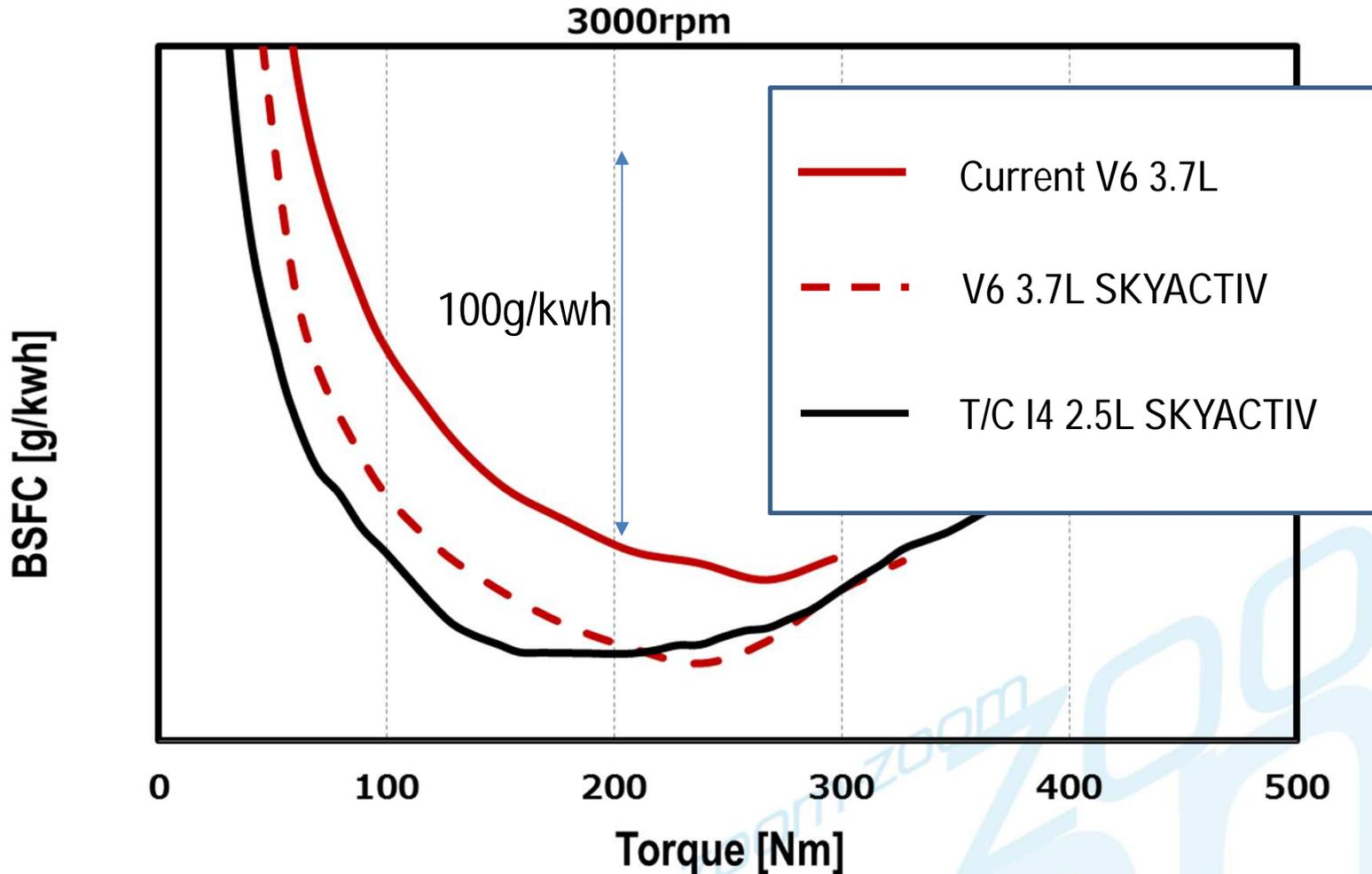
The most efficient way to downsize engines is to convert V engines to inline engines and downsize, while controlling knocking in the high load range with specific technologies to boosted engines.
