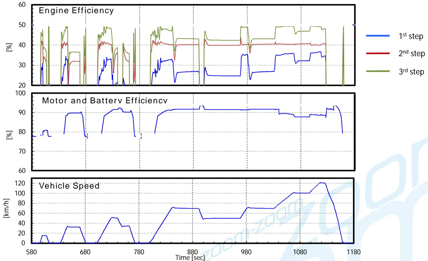
ICE vehicles will be able to attain the CO<sub>2</sub> level of EVs based on mode simulation. Efficiency improvement for EVs is nearing its limit.
