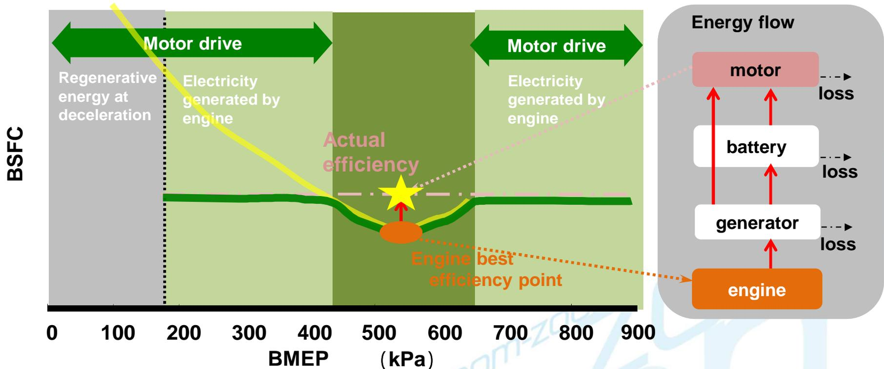
Motor drive using electricity generated by engine = Large battery and large motor required
