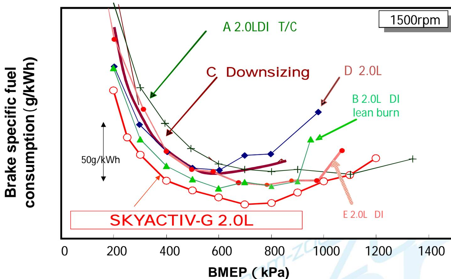
SKYACTIV-G surpasses competitors' all new engines including 30% downsized engines in fuel efficiency.
