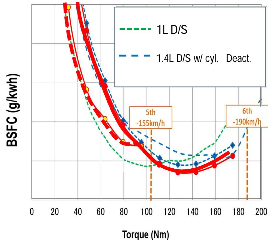
2L SKYACTIV engine can be superior to 1.4L boosted D/S engine with a cylinder deactivation system, and 1L 3 cylinder boosted D/S engine in all operational ranges.
