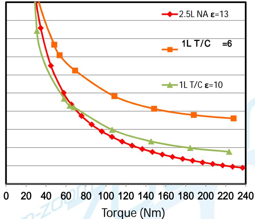
At low load , 1L boosted engine with usual CR=10 shows better BSFC than 2.5L NA, but at mid. and high load, 2.5L engine shows much better BSFC than 1L boosted engine.
